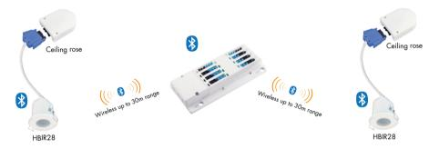
Hytronik's Bluetooth sensor can be plugged to a nearest ceiling rose, without needing to connect a long cable to the QCB03/BLE. This Bluetooth sensor will be able to wirelessly control all the luminaires that are connected to the QCB03/BLE. This is extremely useful by saving long cable wirings when there are multiple Bluetooth sensors controlling a same group of luminaires.
