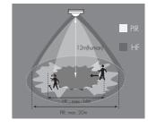
HF detection:  $\emptyset = 14$ m (max.) PIR detection:  $\emptyset = 20m \text{ (max.)}$
