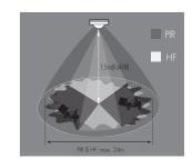
PIR detection:  $\emptyset = 24m \text{ (max.)}$ HF detection:  $\emptyset = 24m \text{ (max.)}$
