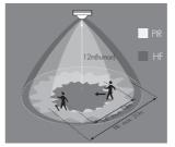
HF detection:  $\emptyset = 14m \text{ (max.)}$ PIR detection:  $\emptyset = 20m \text{ (max.)}$
