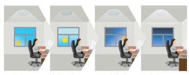
The light turns on at full or dims to maintain the lux level. The light output regulates accroding to the level of natural light available.
