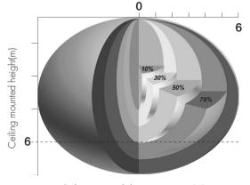
Ceiling mounted detection pattern (m)
