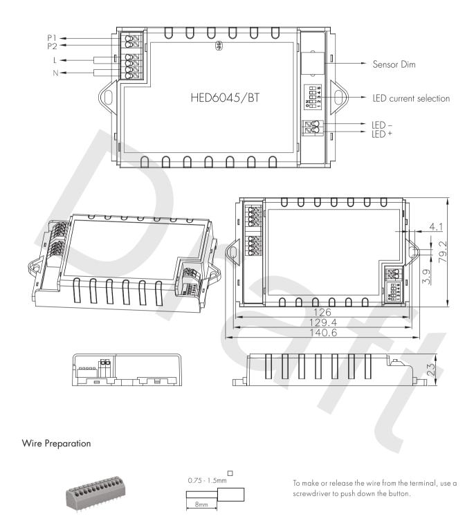
Note: There is no need for any hardwirings on "push" terminal between one driver to another. The installer only needs to connect the push switches to the nearest driver to save labor and cost. The push switches can be assigned to control any Bluetooth driver through the app commissioning.
