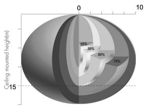
Ceiling mounted detection pattern (m)
