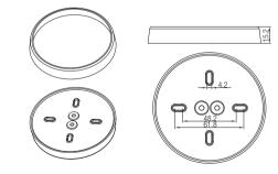
Noted: HIR28/2CH/UH is only suitable for small silicon water-proof gasket
