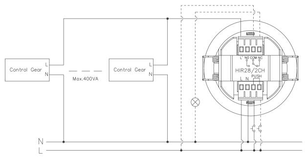
\*By connecting L and COM, the VFC (voltage-free contact) channel can also be turned into a common Switch L output to achieve separate control of the two Switch L channels.
