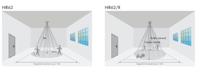
\*The detection patterns are based upon 5km/h movement speed.
