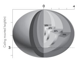
The detection range is heavily influenced by sensor placement (angle) and different walking paces.
