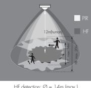
HF detection:  $\emptyset = 14m$  (max.) PIR detection:  $\emptyset = 20m$  (max.)
