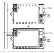
Com Connections (When used together with Hytronik DALI motion sensors)
