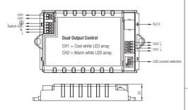
Note: Connecting a sensor antenna will disable the com input on the driver.
