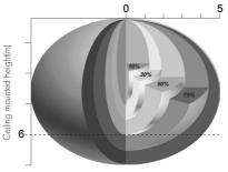
Ceiling mounted detection pattern (m)
