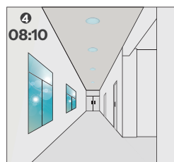
The light turns off completely when natural light lux exceeds daylight threshold pre-set.
