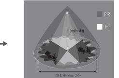
PIR detection:  $\emptyset = 24$ m (max.) HF detection:  $\emptyset = 24$ m (max.)
