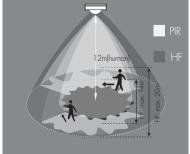
HF detection:  $\emptyset = 14m \text{ (max.)}$ PIR detection:  $\emptyset = 20$ m (max.)
