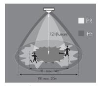
HF detection:  $\emptyset = 14$ m (max.) PIR detection:  $\emptyset = 20$ m (max.)
