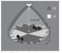
PIR detection:  $\emptyset = 24m$  (max.) HF detection:  $\emptyset = 24$ m (max.)
