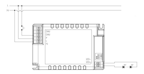
Wiring Diagram For Sensor Dim
