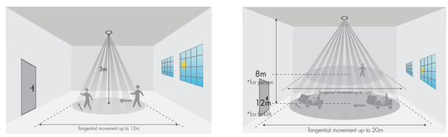
\*The detection patterns are based upon 5km/h movement speed.
