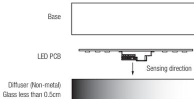
Diagram 2. Typical layout - behind LED PCB with cut-out
