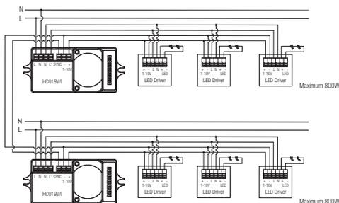
\*Earth if required - (no earth connection necessary on HC019V/I)
